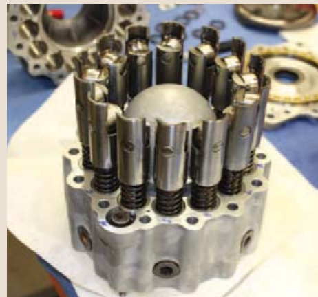
Inside of the fuel injection pump showing the roller plungers
