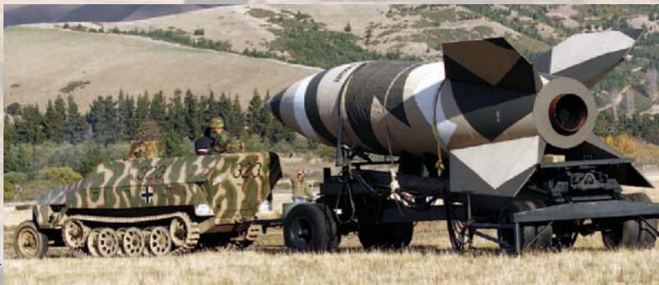
The remarkable full-scale V-2 rocket and the amazingly convincing 'Meillerwagen' trailer were appropriately towed into position by the German Hanomag half-track before the rocket was raised to the firing position.
