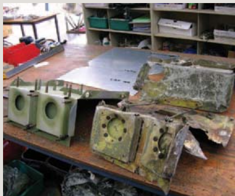
An example of the work required. Here new oxygen bottle mounts are made using the damaged originals as patterns.
