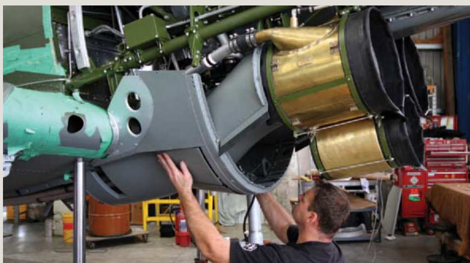
Derek Smith checks the alignment of the cowl flaps.
