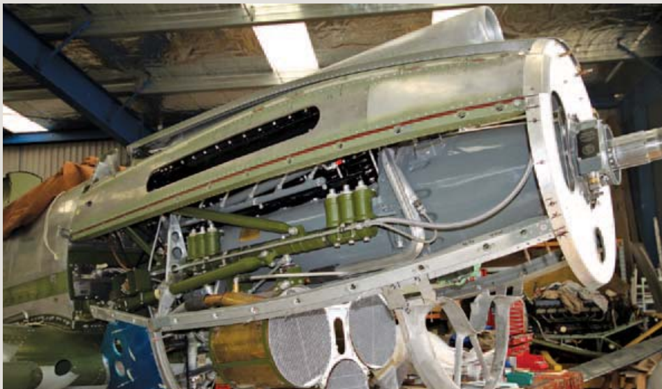
Progress on the complex cowlings, the original inlet casting was repaired for re-use.
