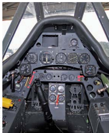
Flug Werk FW 190, ZK-DFR cockpit layout, the missing instrument top left is that of the ammunition counter.
