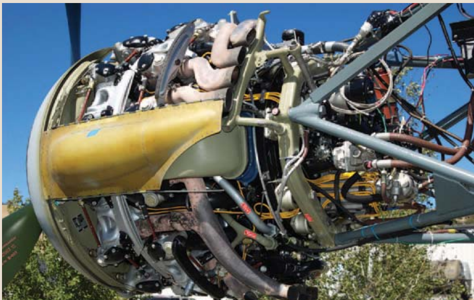
The BMW attached to the custom built test stand where it would stay for three weeks and undergo 10 + hours of run time.
