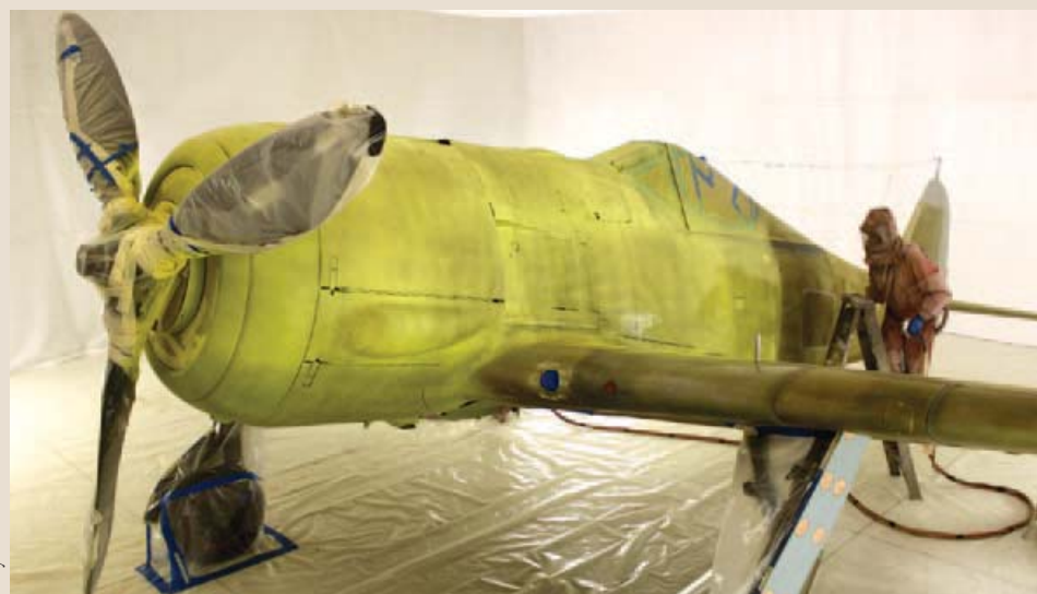
Cocooned inside a custom built paint booth, painting of the aircraft gets underway with Don Copeland of Arizona Aeropainting LLC on the spray gun.
