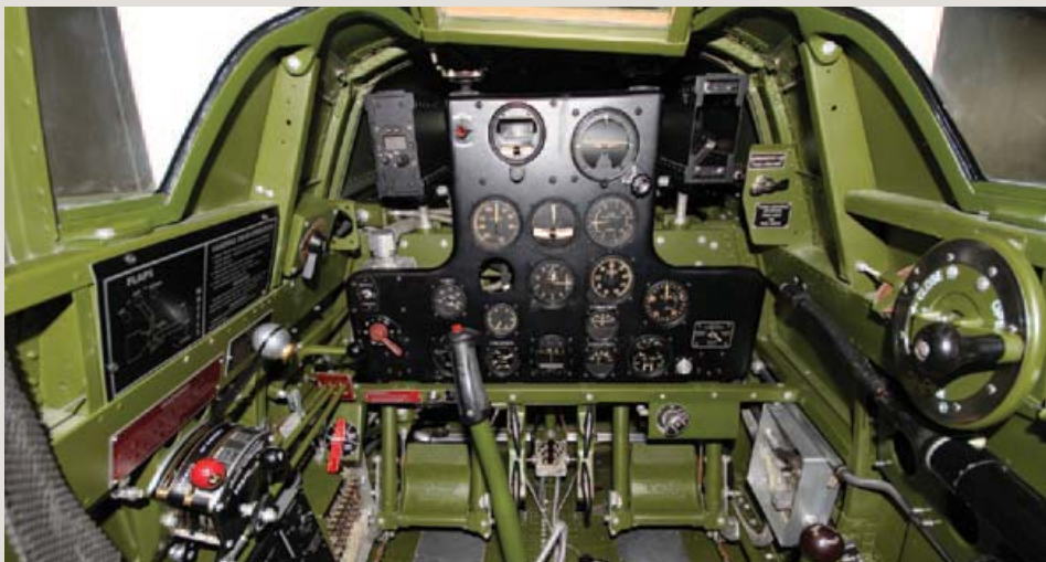
Cockpit shot showing the gun butts removed to reveal the VHF Radio and Transponder installed in the replica 50 caliber machine runs. The Tomahawk cockpit is significantly different from the Kittyhawk.
