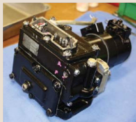
The propeller pitch control unit with the hydraulic and electric motors.
